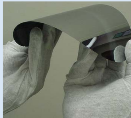
8" SILICON WAFER GROUND TO 120 μm WITH 25 Å RA SURFACE FINISH (NO ETCHING)
