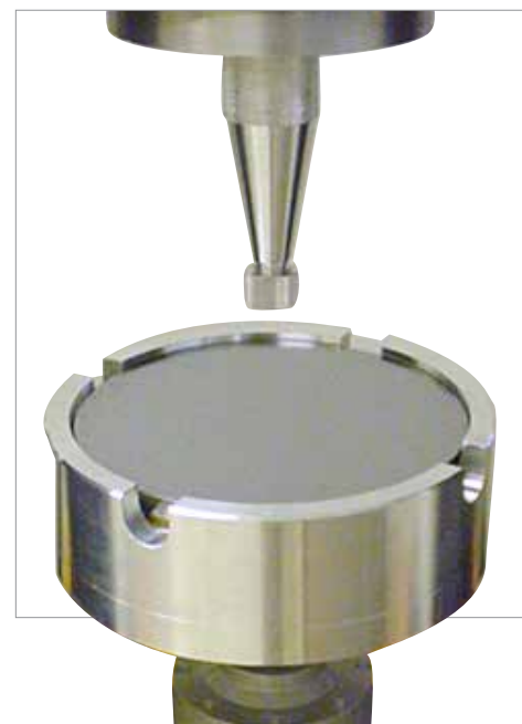
INTERNALLY-DEVELOPED NORTON BALL ON RING WAFER STRENGTH TEST BED
