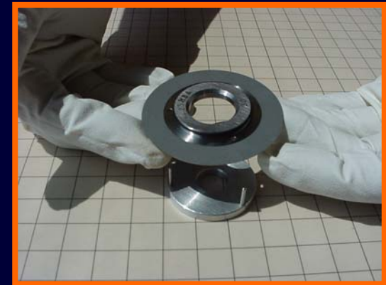
19. Remove used blade and dismounting tool.
