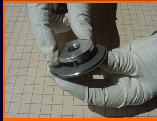
15. Insert dismounting tool in holes.
