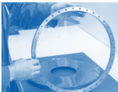
Pict. 8: Clean and degrease upper clamping ring.
