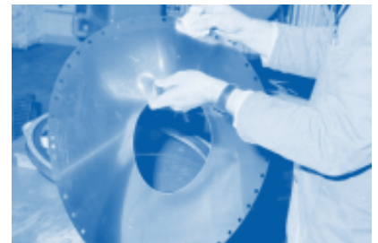
Pict. 4: Clean and degrease clamping areas. -Clean blade tensioning support area and cover the area with a thin coat of lubricant.
