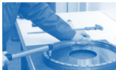
Pict. 11: Tighten clamping screws crosswise using an Allen wrench. Generally the clamping ring screws (M6 property class 12.9) are tightened with a torque wrench to 15 Nm. To avoid screw failure, screws should be replaced at every blade change.
