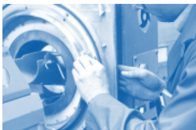
Pict. 12: Clean tensioning ring and cover it with a thin coat of grease.
