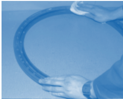
Pict. 1: Remove clamping ring bleed screw and metal tensioning ring. Reinsert bleed screw and tighten it. Clean and degrease clamping ring surface.
