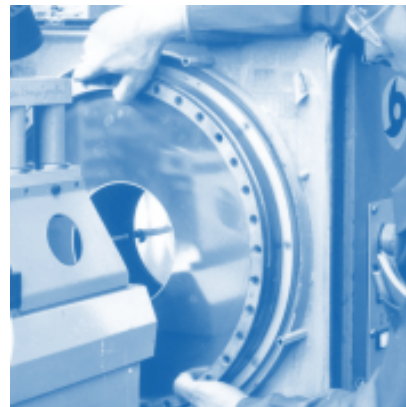
Pict. 13: Mount clamping rings with saw blade on top of tensioning ring.
