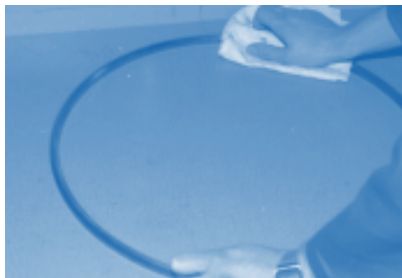
Pict. 2: Clean and degrease the blade clamping areas (on each side) and position the blade on the clamping ring guide pins.
