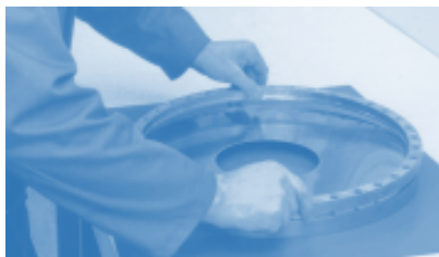
Pict. 9: Match up balance marks of clamping rings and place upper clamping ring properly aligned on top of blade and lower clamping ring.
