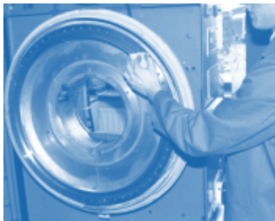
Pict. 3: Clean metal tensioning ring, cover the tensioning area with a light coat of lubricant and insert ring in the clamping ring groove.
